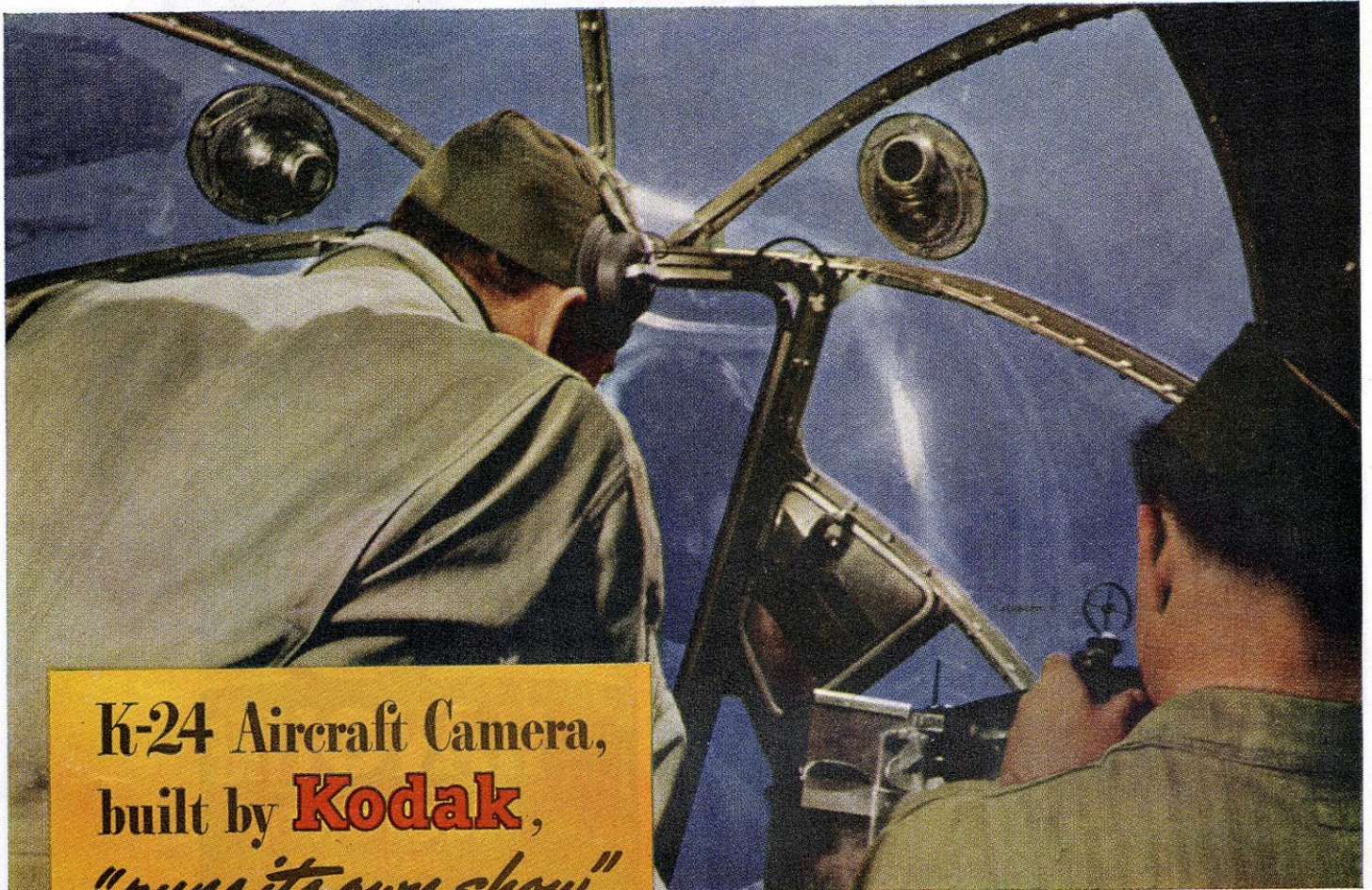
Bombardier, at left, is hunched over his bombsight which is electrically coupled with the camera, automatically taking pictures every time bombs are released. At right is a gunner.
